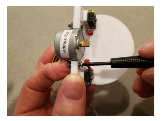
(3) There are two stepper motor driver boards that are mounted on the camera base. Position the driver board with the red switch block in the UP position. Attach the board using two short screws and nuts as shown.
