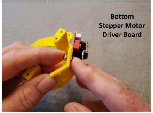
(4) Hold the camera base and driver board with the red switch block facing as shown. Hold the nut in place with your finger on the screw holding the assembly in place. Carefully place a nut on the screw turning the screw in a clockwise. Install the second screw. Gently tighten both screws to complete the assembly. Attach the second stepper driver board using two short screws as shown.
