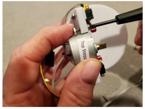
(2) Fit the second screw and nut to secure the other side of the stepper motor. Note that the stepper motor is mounted on the same side as the limit switches.
