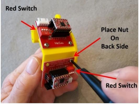
(5) The camera base with both driver boards should appear as shown. The left board controls the bottom stepper motor, and the right board controls the top stepper motor.
