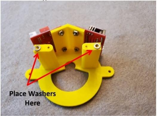
(7) Place a stepper motor on the camera base as shown. The motor wires are routed behind the motor. Both stepper motors are the same.Note: The placement of the washers.
